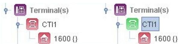
**Figure 9** Left: Unregistered Media Terminal; Right: Registered Media Terminal
